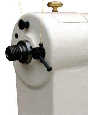
in a plate in the headstock. When the pin locks in place drop the lever into the second slot to keep the spindle locked in place.
