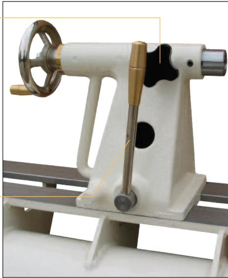
**Installation of Accessories:** To install an accessory in to the tailstock, wind the barrel out 1". Put the accessory in the barrel, and snap it into the taper.
