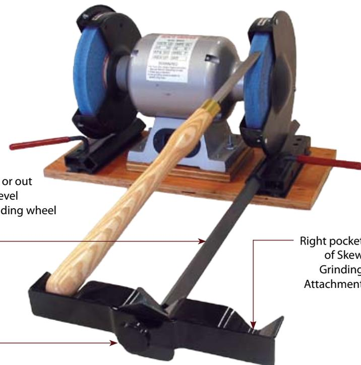
VEE-ARM: adjust this in or out to match the existing bevel of your skew to the grinding wheel
