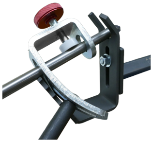
The 4th notch is recommended for bowl gouges
