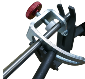
The 2nd notch is recommended for spindle gouges
