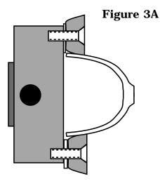
Here we show how you can hold objects with a minimum diameter of 3/8" with the buttons mounted on the inside holes and up to a maximum diameter of 3" with the buttons mounted on the outside holes.
